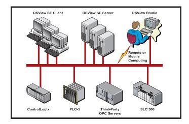
Supervisory-level applications are deployed on RSView<sup>®</sup> SE<sup>™</sup> Servers, which detect events, manage alarms, collect and process data, and handle other runtime processes.
