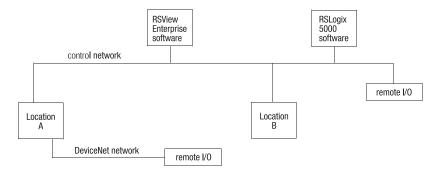
For Location A, if the supervisory network is EtherNet/IP, use a 1769-L32E, -L35E controller because it can share data with the other devices on EtherNet/IP and can simultaneously support EtherNet/IP and DeviceNet communications. Or if the supervisory network is ControlNet, use a 1769-L32C, -L35CR controller.
