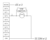
Most output modules have built-in surge suppression to reduce the effects of high-voltage transients. Use an additional suppression device if an output is being used to control inductive devices, such as relays, motor starters, solenoids, or motors. Additional suppression is especially important if your inductive device is in series with or parallel to hard contacts, such as push buttons or selector switches.
