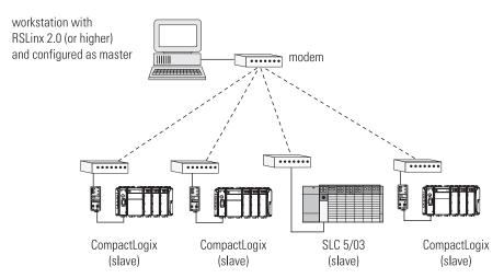
If you connect the controller to a non-isolated port (channel 1) on the controller to a programming workstation, modem, or ASCII device, install an isolator between the controller and the end device. One possible isolator is the 1761-NET-AIC interface converter.
