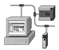
RSNetWorx software is the configuration tool for your control network. With RSNetWorx software you can create a graphical representation of your network configuration and configure the parameters that define your network.
